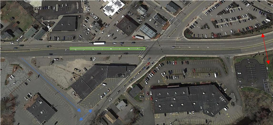
Solutions may include some reconfiguration of the intersection and traffic flow. This might include repositioning right and left turns from the eastbound lanes to Mah Way (blue arrows) and adding a landscaped center lane in place of the existing turn lane (green rectangle), moving overhead utilities underground, and buffering sidewalks from vehicular traffic.
