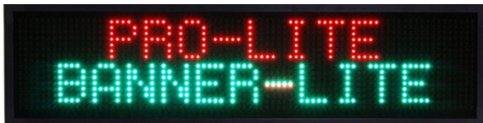
Figure 18: Electronic Variable Message Sign
