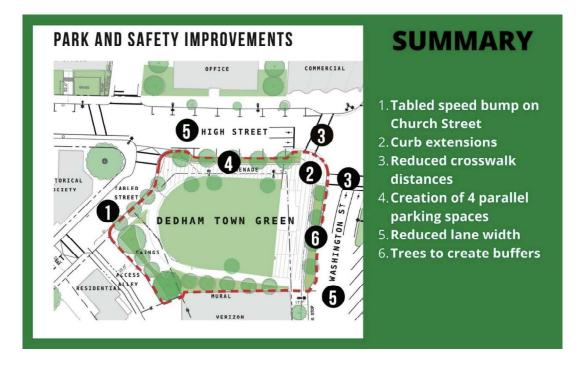
In preparing the concept design, Mr. Giard looked for ways to increase the safety of the existing intersection at Washington and High Streets, working with the Town Engineer to ensure improvements would not reduce the current Level of Service (LOS) of the intersection. The above plan highlights specific streetscape changes proposed, which would improve pedestrian safety and increase the amount of usable park space by about 15%.
