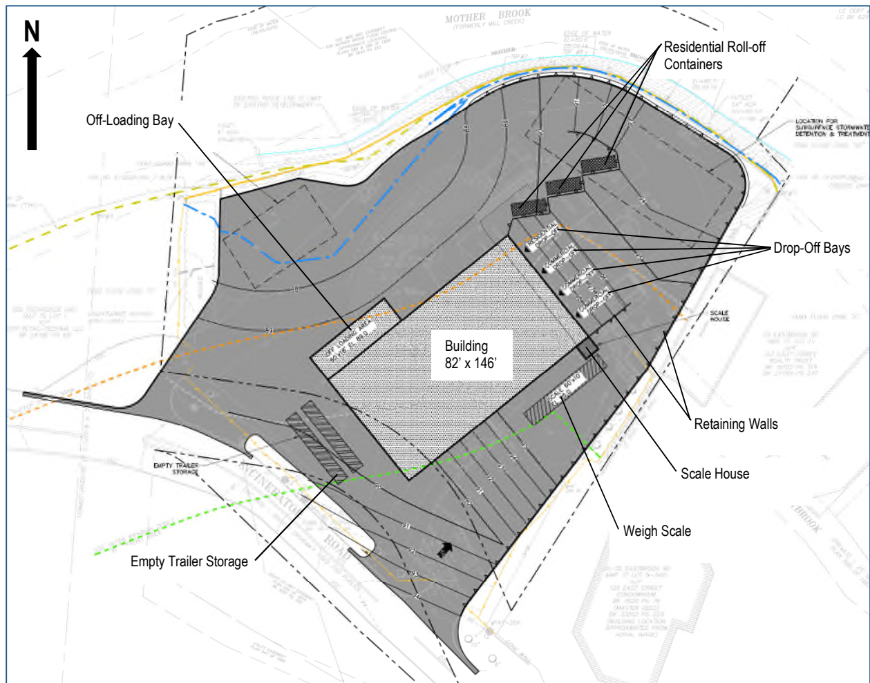
Figure 3-3: Transfer Station Alternative Site Layout B
